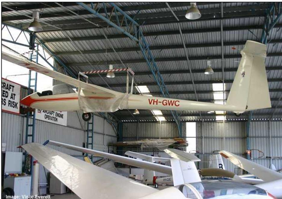
Seen here in its storage cradle at Caboolture is the ICA-Brasov IS-29D VH-GWC now in possession of QAM. A high performance sailplane it represents the first Romanian designed and built aircraft in the Museum's collection. With a 15m (49ft) wing span it weighs only 240kg (529lb) empty. (Photo- Vince Everett)
