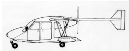
Fig 2 A possible appearance of the aircraft if it had been completed with a Franklin 125hp engine (Del IW). The fairing below the engine is assumed to be similar to that of the Marchetti Riviera which tapers to a point. Aerodynamically it cannot end abruptly
